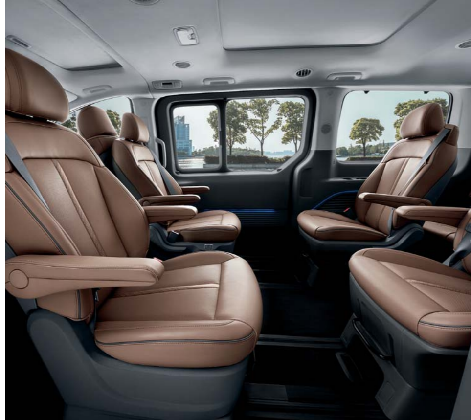
Swiveling independent seat STARIA Premium's flexible seating multiplies the fun factor, especially when traveling with children on long-distance trips. The 2nd-row swiveling independent seat rotates 180° degrees to allow face-to-face conversation among rear seat passengers and 90° to promote easier entry and egress.
