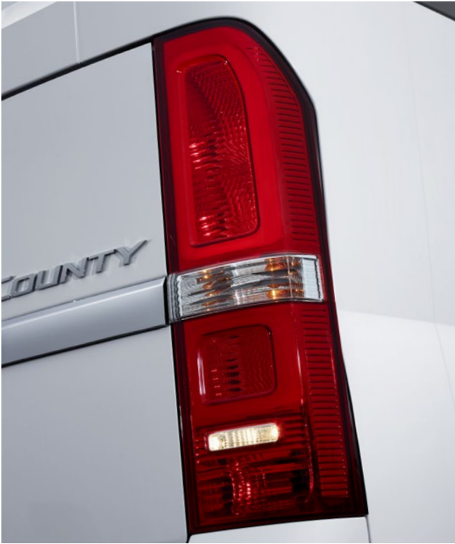
Vertical Rear Combination Lamps Standing tall and proud, the new vertical-style tail lights provide maximum visibility and allow the enlargement of the cargo flap door to improve access to the luggage space.
